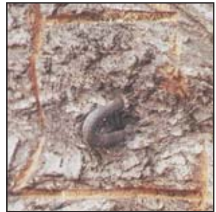
The metal object in this log has been clearly marked to indicate its presence.
